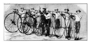
The 'ordinary' in turn evolved during the 1880s into the 'safety' bicycle where chain drive to the rear wheel allowed the front and rear wheels to be of equal size, dramatically reducing the risk to the rider of pitching over the handle bars. It also enjoyed the comfort of the pneumatic tyre.
